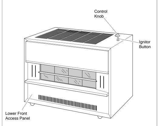
Figure 1 - Vented Propane Gas Heater
